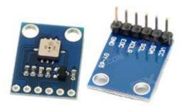
Figure 4. BMP085 barometric presser sensor
