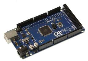
Figure 2. Photo of Arduino Mega 2560 microcontroller board
